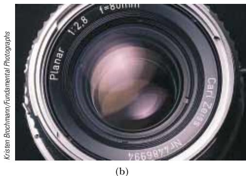
Figure 37.20 (Example 37.4) (a) Reflective losses from a silicon solar cell are minimized by coating the surface of the cell with a thin film of silicon monoxide. (b) The reflected light from a coated camera lens often has a reddish-violet appearance.
