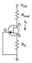
**Source Follower.** The simple source follower is shown below. The improved version is shown at the right. The lower JFET forms a current source. The result is that  $V_{GS}$  is held constant, removing the defects of the simple circuit.
