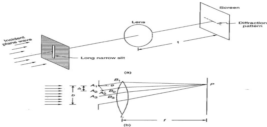
Fig- 1: Diffraction in a single slit.
