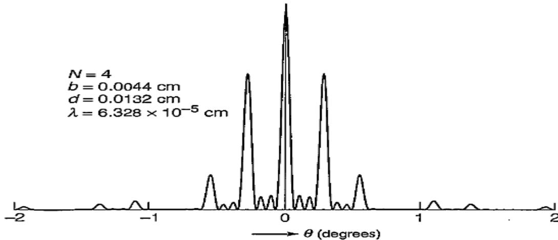
Fig. 5 - The intensity distribution corresponding to the four-slit Fraunhofer diffraction pattern as predicted by Eq. (50) corresponding to  $b = 0.0044$  cm,  $d = 0.0132$  cm and  $\lambda = 6.328 \times 10^{-5}$  cm. The principle maxima occur at  $\theta = 0.275^\circ, 0.55^\circ, 0.82^\circ, 1.1^\circ, \dots$ . Notice the (almost) absent third order.
