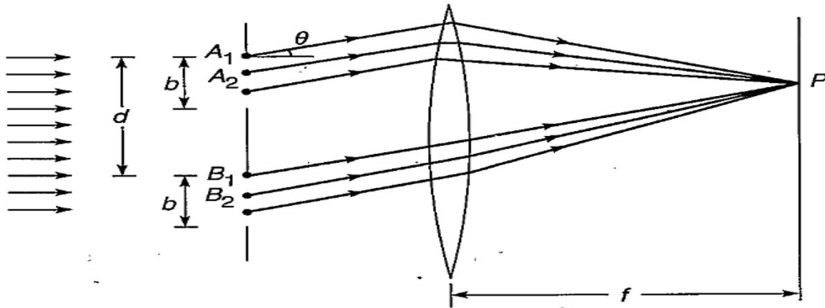
Fig.2 – Fraunhofer Diffraction in a double slit
