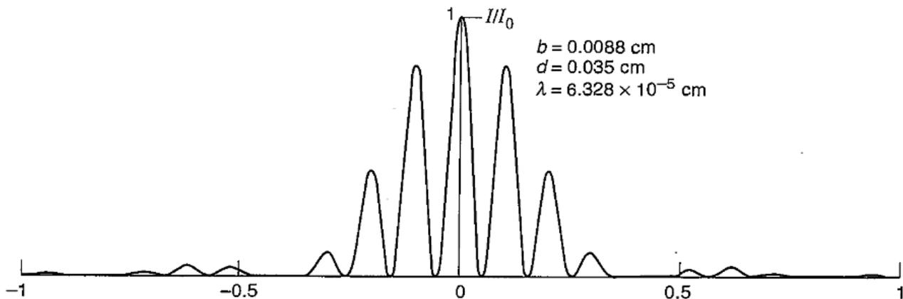
Fig.3 - Intensity distribution pattern due to double slit
